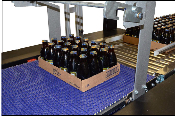
Figure 2-4 - In-feed to Acceleration Conveyor
