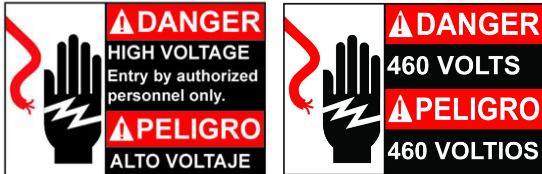
Figure 1-1 - Red & Black labels indicate DANGER hazards
